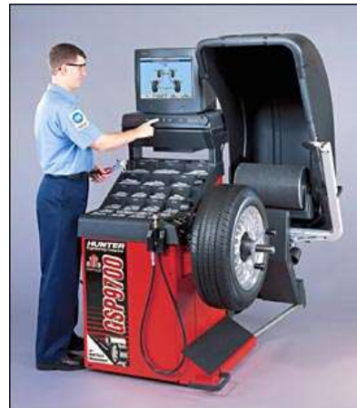
FIGURE 9.10 Two-plane balancing. (Courtesy of Bruel and Kjaer Instruments, Inc., Marlborough, Mass.)
